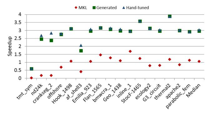
Fig. 8. Speedup of Parallel PCG over Sequential PCG.
